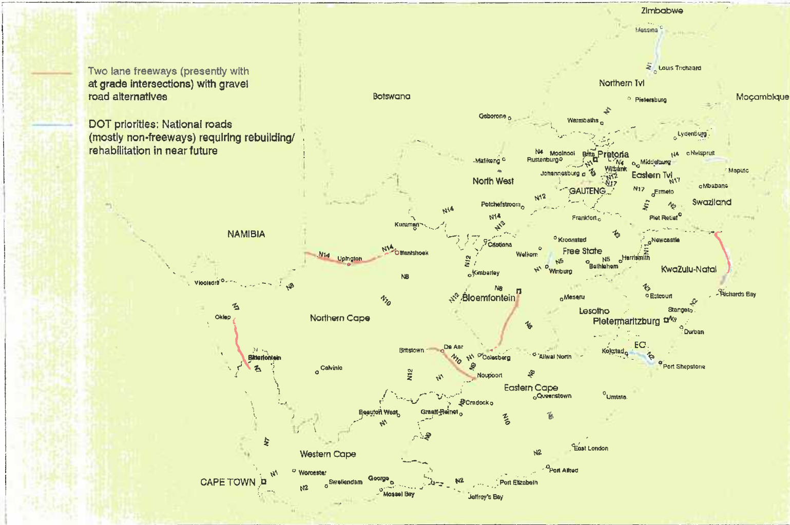
Freeways with gravel alternatives and non-freeways requiring rebuilding/rehabilitation
